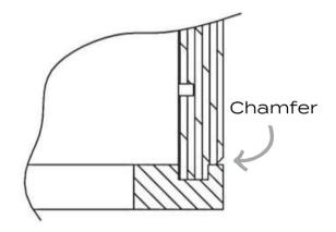
1/2" Finished Plywood Integrated End Panels
